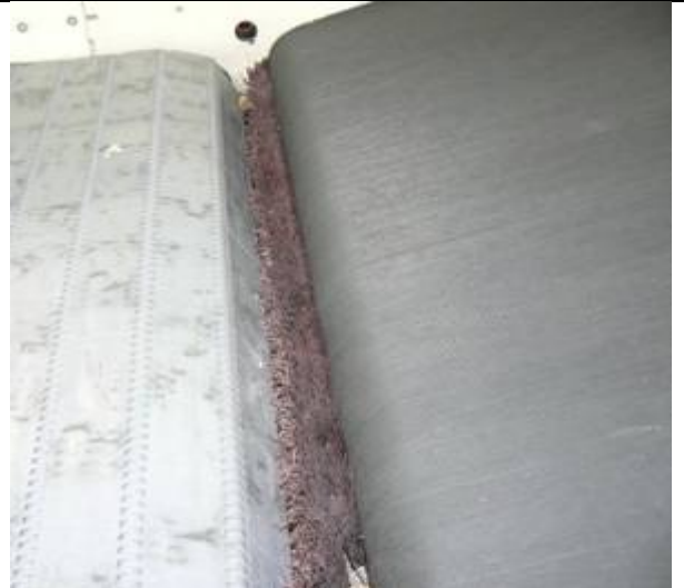
Illustration 18: Modification of the other APPS machine with a broom-type sweep eliminates parcel damage and slip-through.
