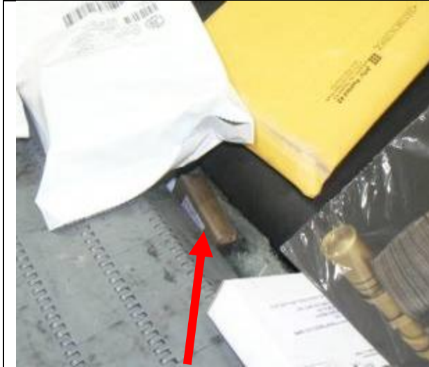
Illustration 17: Small package damaged in space between APPS feeder belts.
