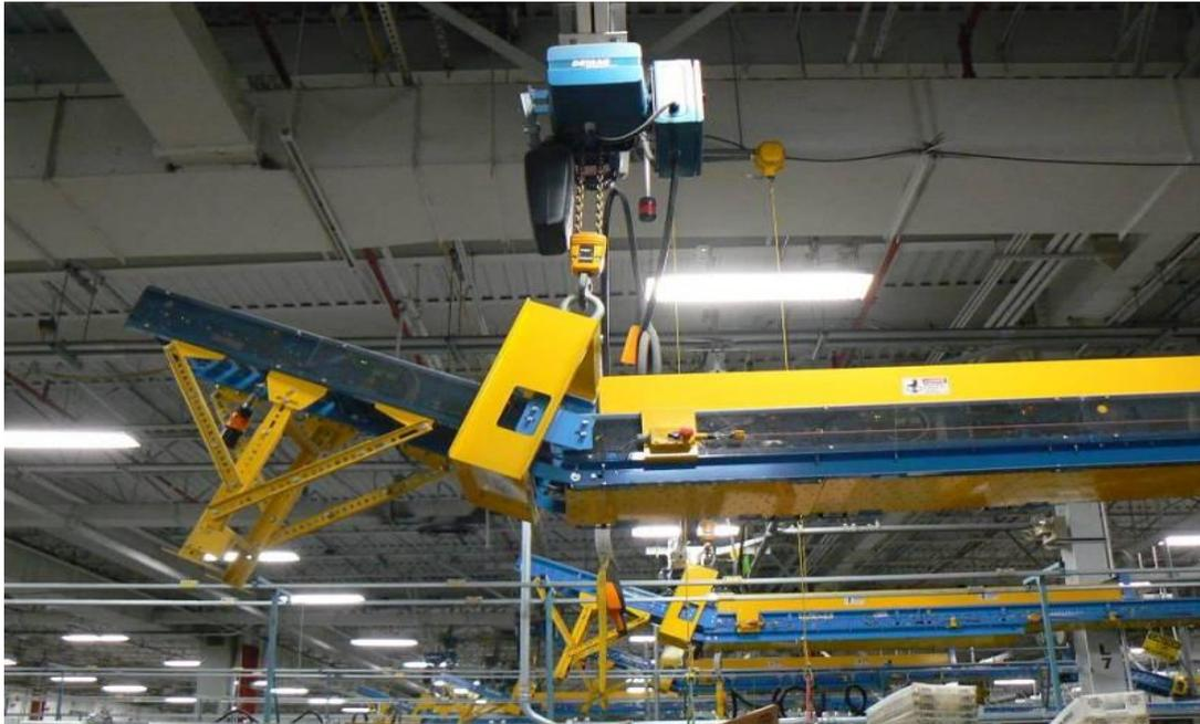
Source: OIG, *Efficiency Review of the Cleveland OH Processing and Distribution Center* (Report Number NO-AR-12-005, dated June 5, 2012). The tray takeaway system located at each Delivery Barcode Sorter has not been used for more than a year. Using this system would reduce mail processing times.
