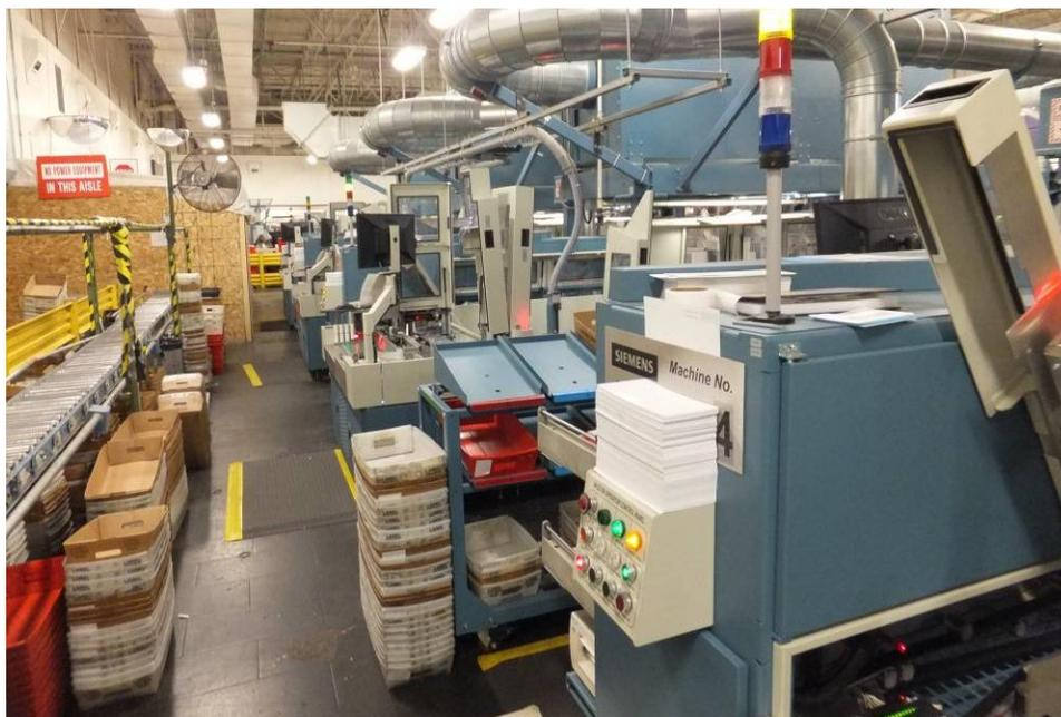
Source: OIG photograph, dated June 26, 2012. Cancelled letter mail from the Automated Facer Cancellation System is trayed and placed on the rollers, where they must then be loaded on rolling stock and moved to the next operation.
