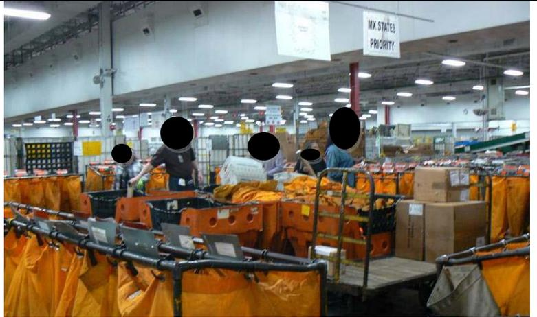
**Picture 8: An employee sorting machineable letters in the manual flat operation. Processing these letters on automation equipment would be more efficient. Source: OIG, January 11, 2012, 9:14 p.m.**
