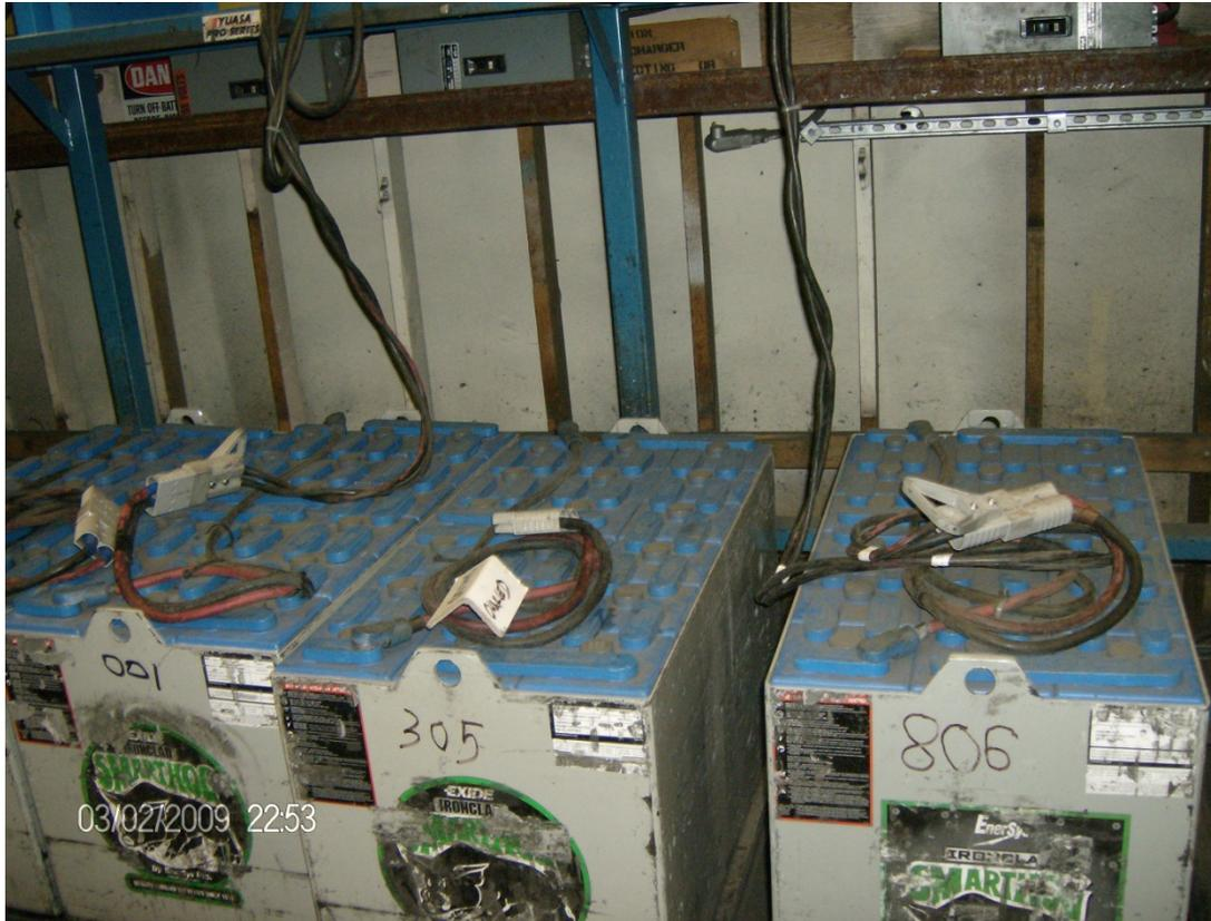
Illustration 1: Batteries did not include battery fobs, which should be located on top of the batteries.<sup>7</sup>
