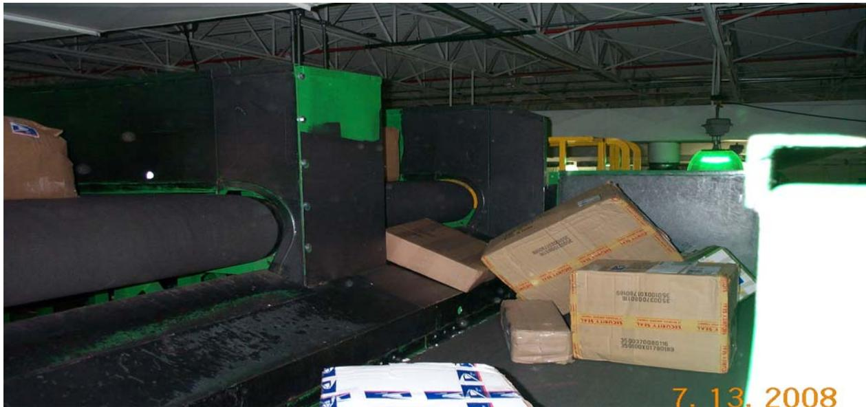
**Picture 2: Mail Damaged After Going Through a Drop-Off Point on a Conveyor System**
