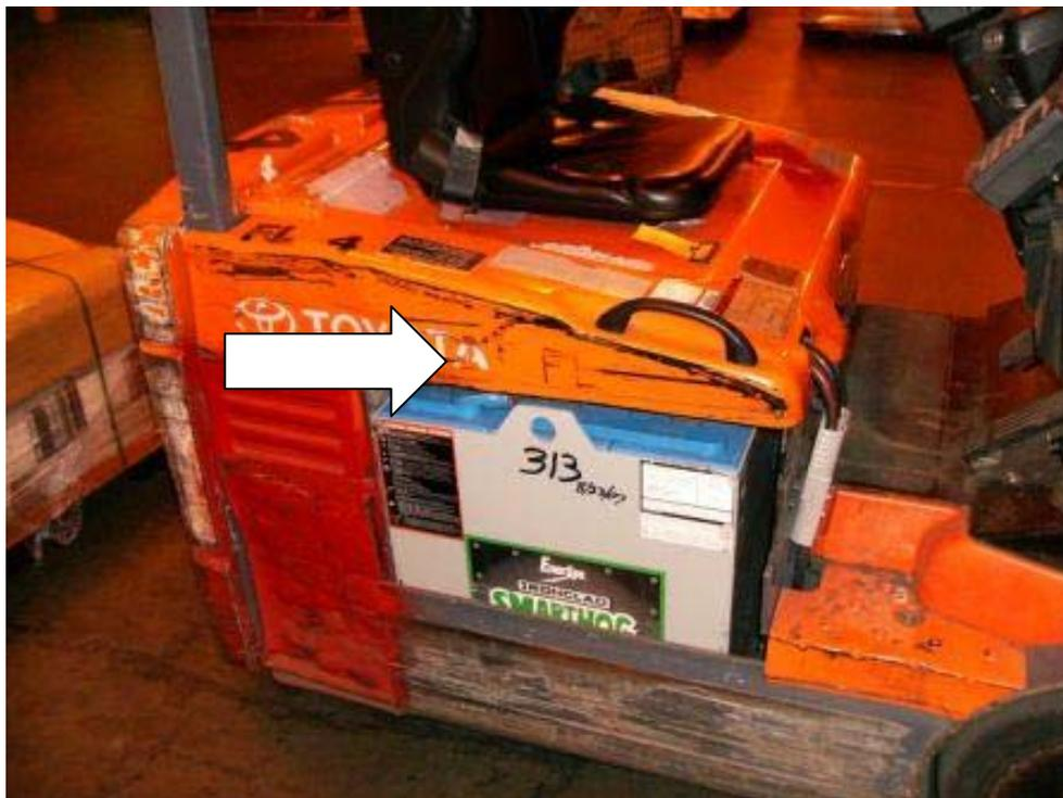
Illustration 3: On April 28, 2008, at 2:20 p.m., we observed a damaged forklift. The side cover was torn.
