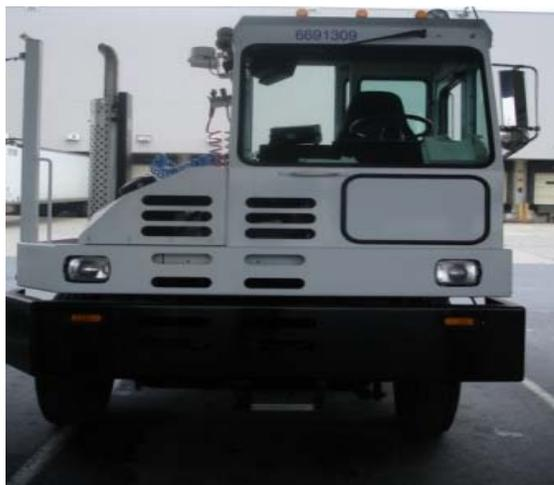
At the Washington NDC, as with all NDCs, PVS assets, such as this spotter tractor, are primarily used for yard operations.
