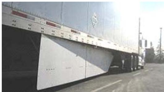
Figure 2: Example of side fairing (trailer skirt): a durable, flexible, and lightweight wind deflector. Freight Wing product shown.
