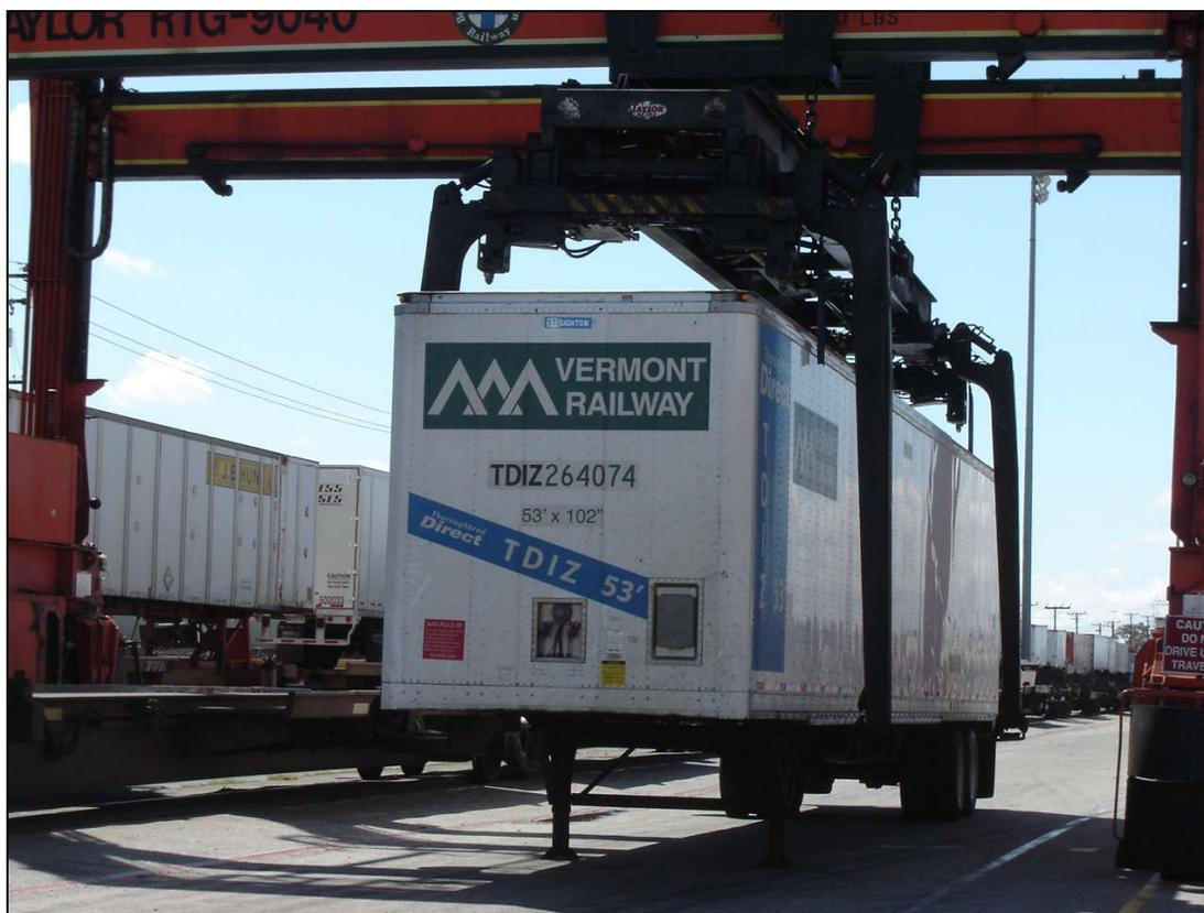
**Highway trailer being lifted onto rail flat-car for rail transportation.
