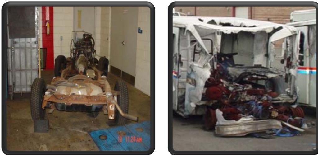
**Vehicles are being completely reassembled to include frame, engine, transmission, and body shell. Available data shows 613 vehicle frames were replaced in FY 2008 and 2,250 frames in FY 2009.**
